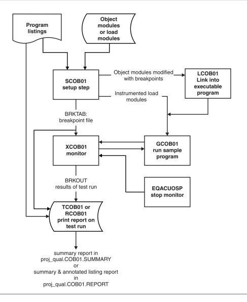
**JCL member names:** The JCL member names for the steps, such as SCOB01, depend on the sample that you are running. For example, the setup JCL for the PLI01 test case is SPLI01.
