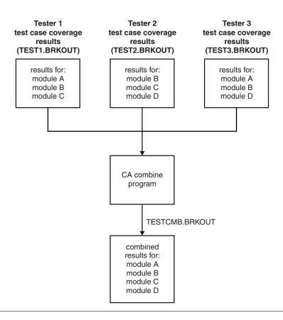
The diagram shows three test case coverage runs that were made, each with a different set of test cases:
