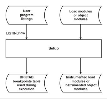
**DD names:** The names outside the box in the figure (for example, LISTINP) correspond to the DD names for the listings.
